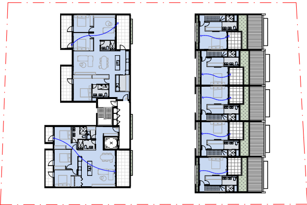
CROSS VENTILATION DIAGRAM - LEVEL 2 1:200
